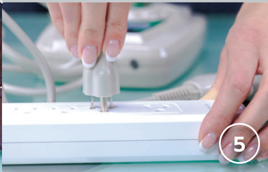
5 Plug the other end of the controller into the power outlet. We suggest to always use a surge protector.
