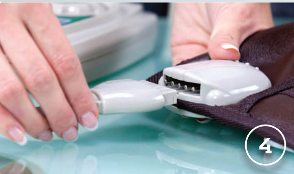
4 Plug the controller into the mat's power port.
